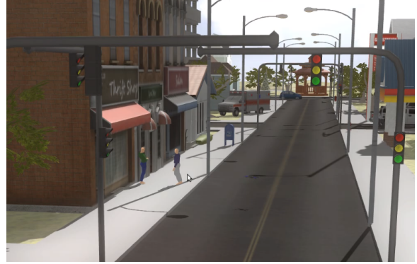
Fig. 3. ROS Gazebo Simulation Environment, combining the Gazebo vehicle and city simulation environment, and the Pixhawk PX4 Flight controller.
