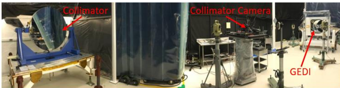
Figure 15: GEDI collimator setup with the GEDI Optical Bench on a white GSE dolly
