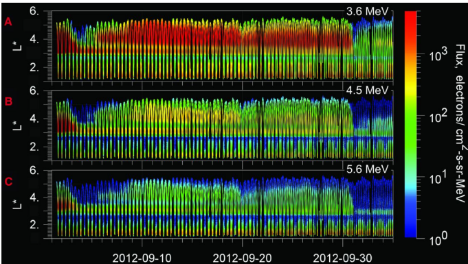
Fig. 1. REPT measurements of energetic electrons showing the electron storage ring (reproduced from [24]).
