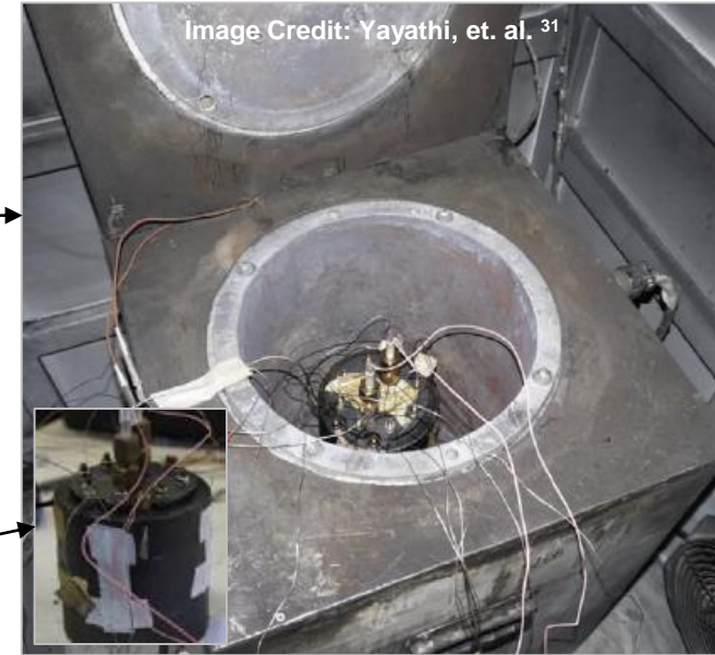
Image above taken from combination ARC-Bomb testing conducted for NASA by Thermal Hazard Technology. Cells characterized included the Boston Power Swing 5300, Samsung 18650-26F, and the Molicel 18650-J
