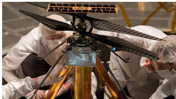
Figure 1 Members of the NASA Mars Helicopter team attach a thermal film to the exterior of the flight model of the Mars Helicopter. 24
