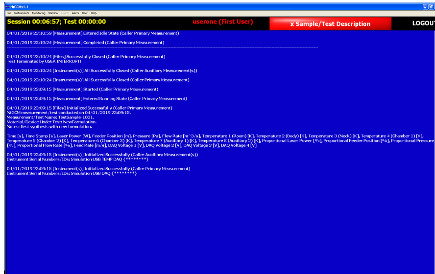
Figure 12: The Measurement Messages Window showing a snapshot of typical messages displayed during a run. These messages will change depending on the communications between the program and the instruments. Note: In the electronic version of this manual, it is possible to zoom in and read the messages displayed in this test instance.
