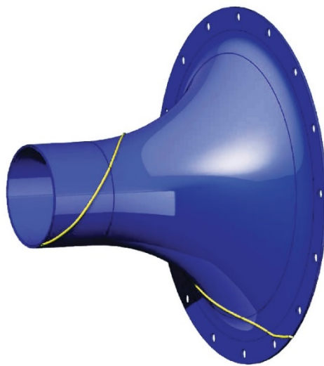
Figure 9.—Load continuity of biaxial braid tow in extended composite section of hybrid gear.
