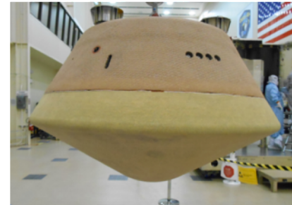
OSIRIS-REx forebody TPS. (~0.8m diameter)
