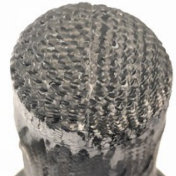
IHF 3": Hot Wall Heat Flux: 3600 W/cm 2 Pressure: 5.3 atm
