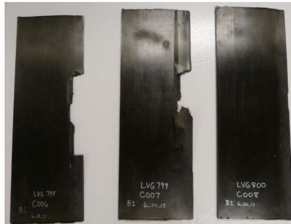
Figure 7: Post-impact images of baseline and TPU toughened blades
