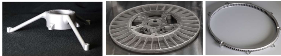
Figure 12: Additively manufactured metallic structural motor components include the housing (left), rotor (center), and finned stator cooling ring.
