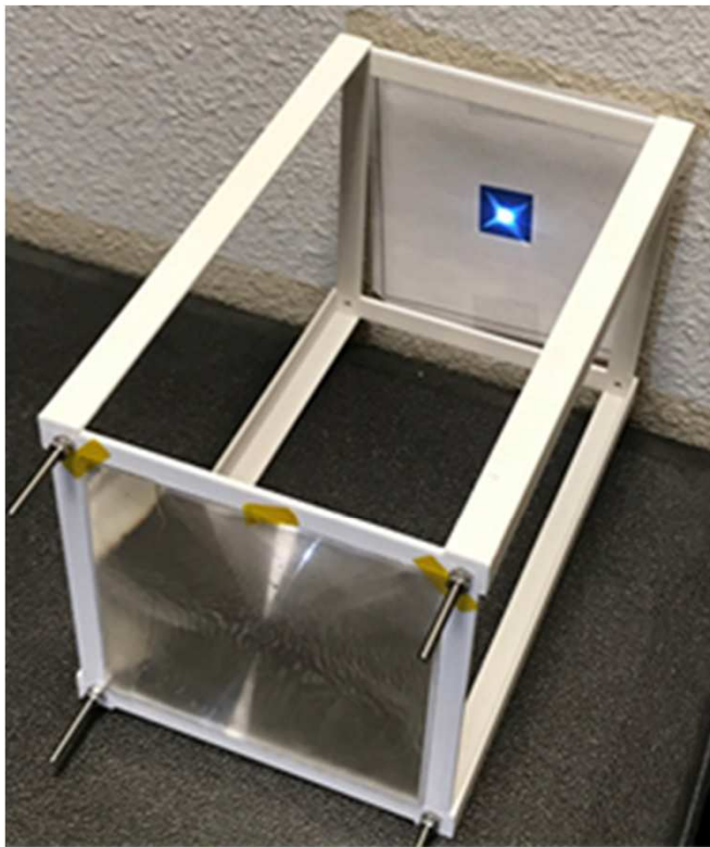
Lens with Thin Ceria-Doped Glass Superstrate
