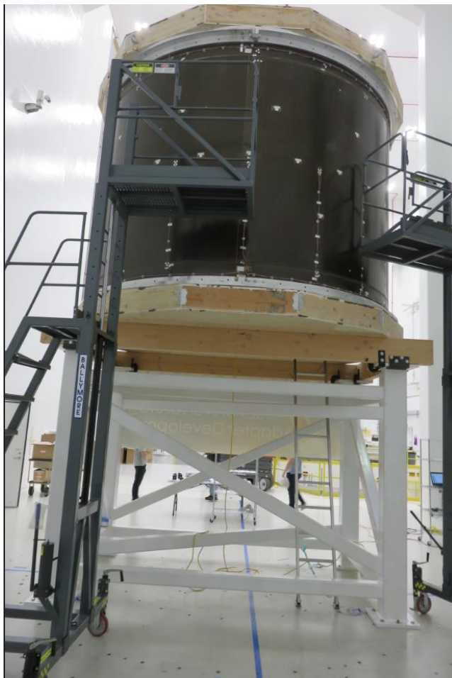
On acoustic test stand (Fixed-Free)
