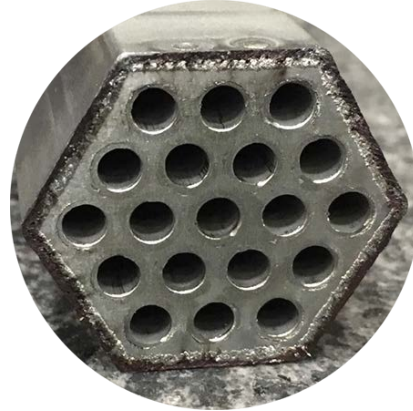
End cap – packed powder fuel element cartridge
