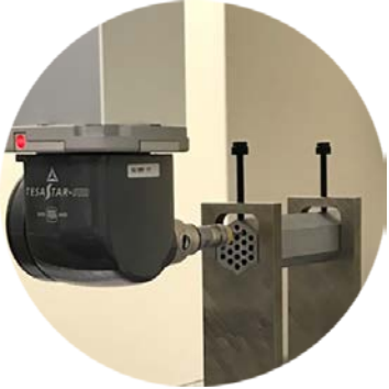
Channel drilling for packed powder cartridge fuel element
