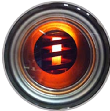
Fuel specimen testing in the MSFC Compact Fuel Element Environmental Test (CFEET) system
