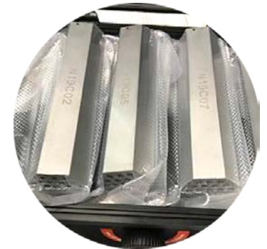
Fuel element packed powder cartridges prior to butt weld assembly
