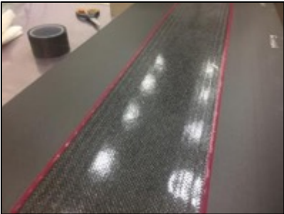
Composite Doubler Following Lay Up and Installation
