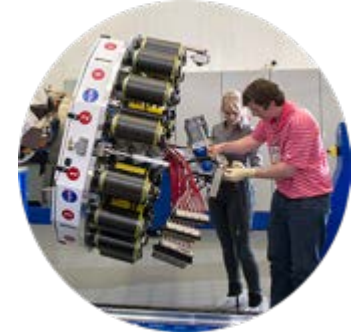
Caption: Replacing tape on the automated fiber placement machine
