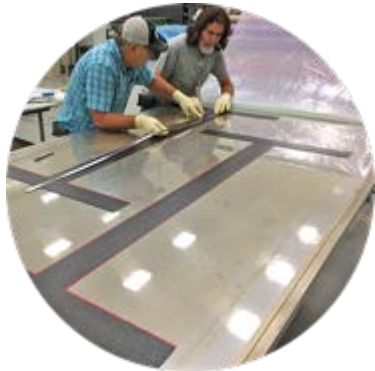
Caption: Layup of a longitudinal composite joint panel
