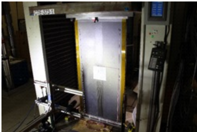
Panel Buckling Test Set-up
