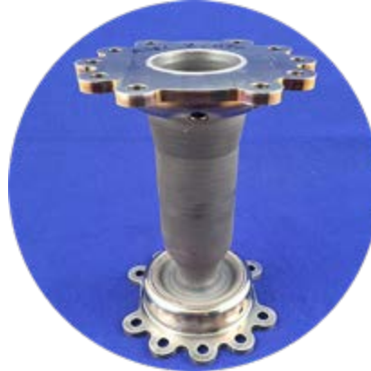
Caption: 1.2K GRCop Thrust Chamber with Composite Overwrap
