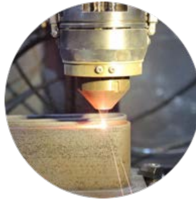
Caption: Initial trials show feasibility of JBK-75 being built using Directed Energy Deposition (DED) process.
