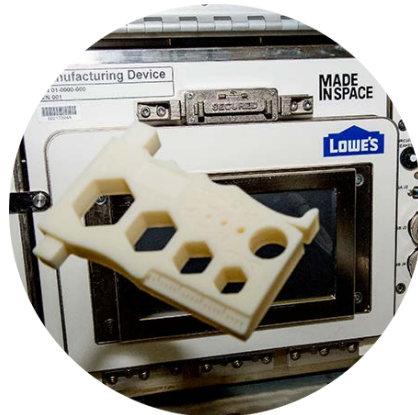
Caption: Future Engineers student-designed part (first student-designed part printed in space!) in front of the commercial Additive Manufacturing Facility
