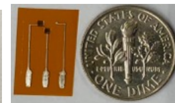
Printed cortisol sensor
