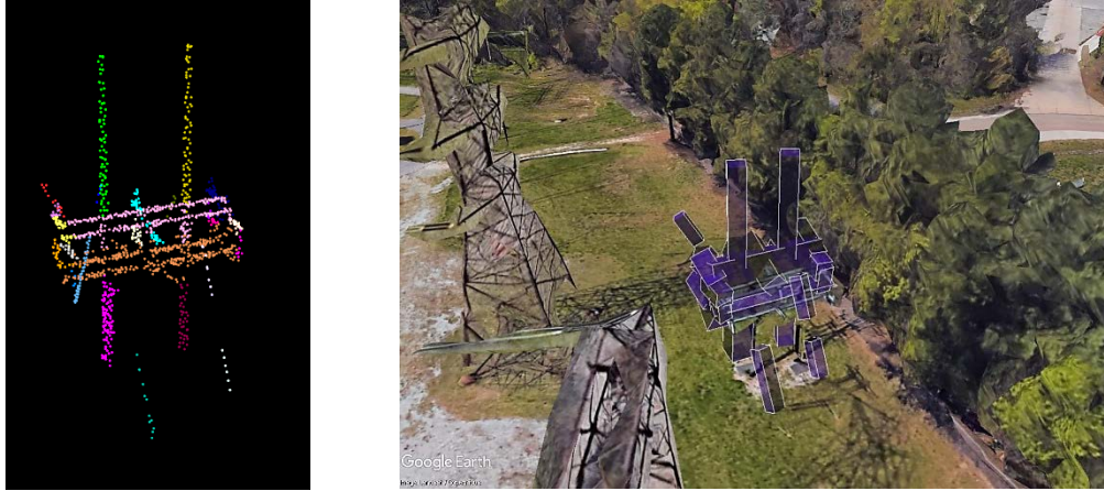
Figure 7. Aerial lidar scans fail to adequately sample fine structures such as guy wires. The 3D Bounding Cylinder method attempts to bridge gaps in sampling by projecting 1 meter along a given cylindrical eigenaxis to search for points in neighborhood construction. If there are no collinear points within a meter, a guy wire with drops in scan sampling is represented as more than one neighborhood (left), yielding multiple bounding polyhedra for the span (right). © Lidar data: Dominion Energy; Map data: Google & DigitalGlobe
