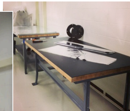
Reflector Layers: Mylar and Kapton cut into rectangles for the blanket cylinder and gore sections for the blanket domes.
