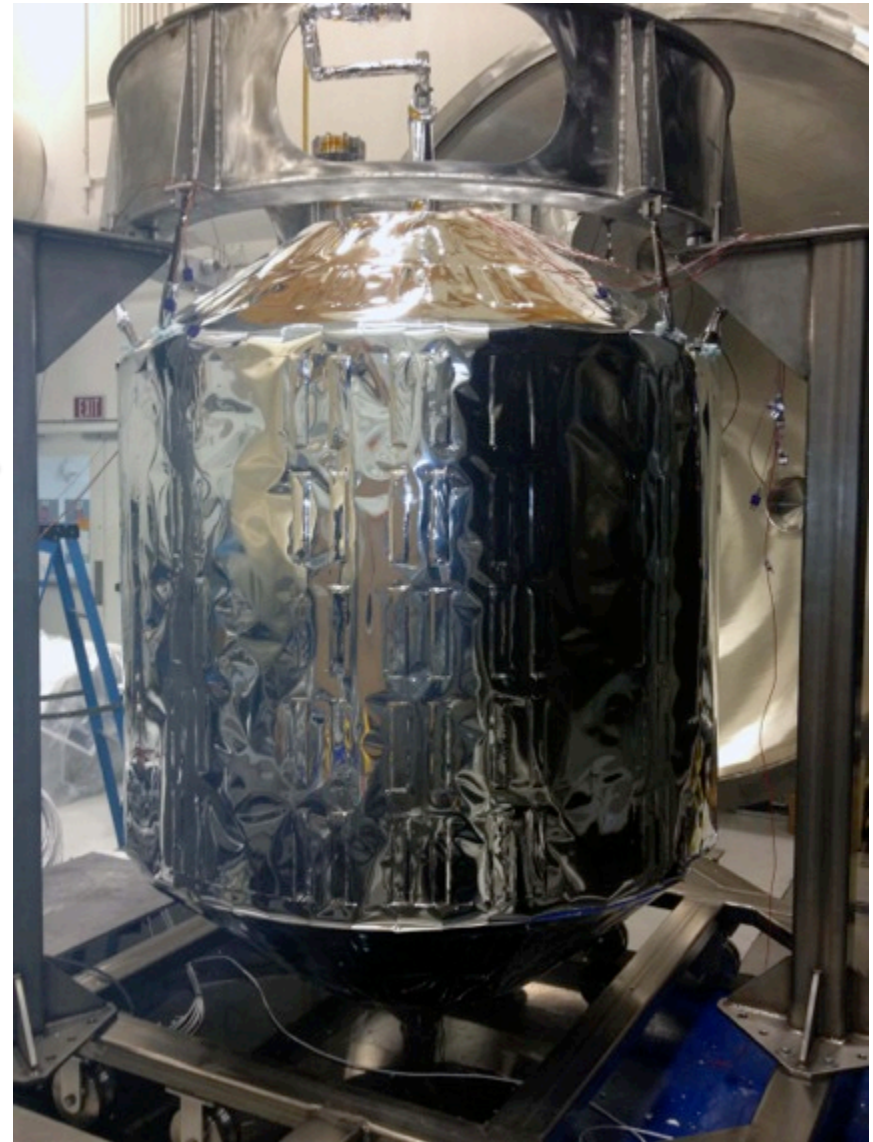
VATA 2d Thermal Test ■ 19-Layer LBMLI
