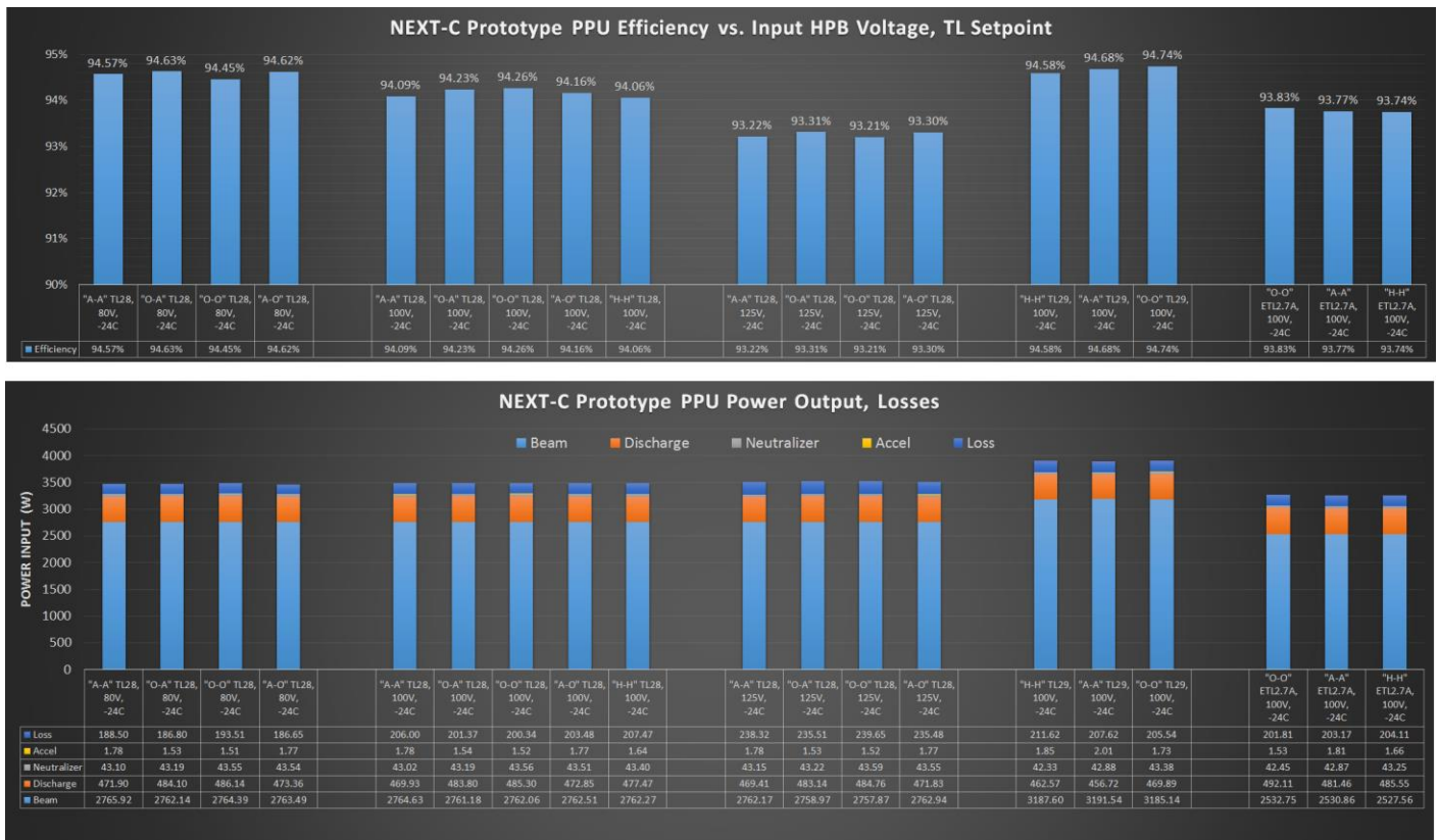
Figure 16. PPU high power bus efficiency, -24 °C baseplate temperature.
