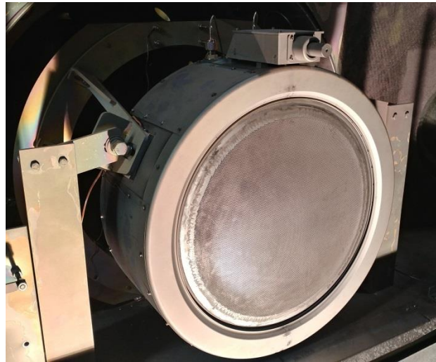
Figure 1. Dev-C engine mounted in VF-16 prior to pump down.
