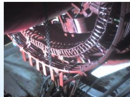
Visual and IR Images of End Winding
