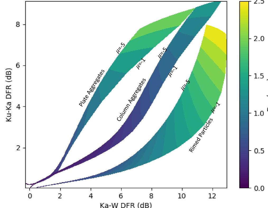
Lookup tables of radar reflectivity ( $Z_{HH}$ ), differential reflectivity ( $Z_{DR}$ ), specific differential phase (KDP), and attenuation ( $k_{ext}$ ) were constructed for each of the three particle families considered. These were integrated over gamma size distributions with a range of mean mass-weighted diameter ( $D_{m}$ ) and shape parameter ( $\mu$ ) shown above.
