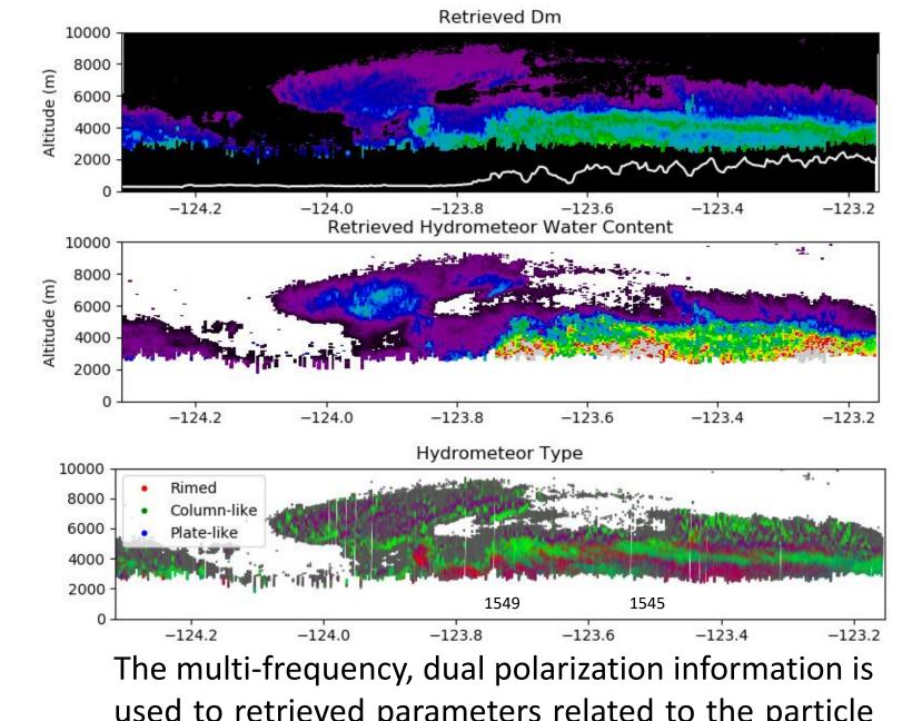
The multi-frequency, dual polarization information is used to retrieved parameters related to the particle size distribution ( $N_{\rm w}$ , from which  $D_{\rm m}$  and water content can be inferred for an given observed Ku dBZ), as well as the partitioning of ice hydrometeors into plates and plate aggregates, columns and column aggregates, and rimed particles, confirmed by in-situ particle probes on the Citation aircraft.
