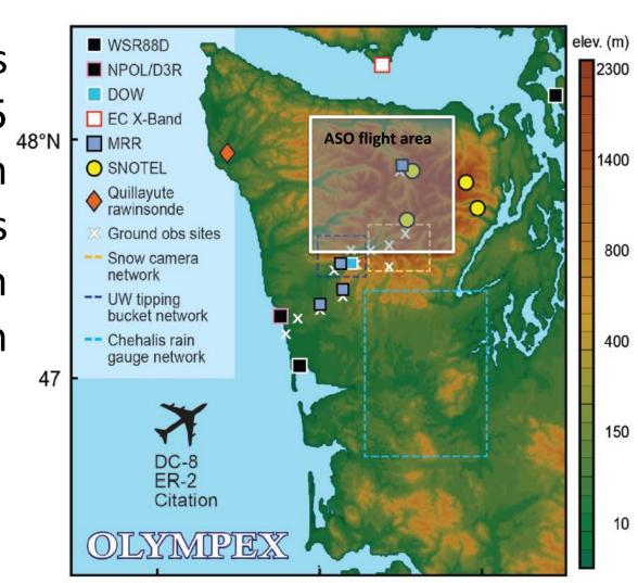
addition to ground sites equipped with disdrometers, remote sensing assets included ground radars (S-band NPOL, C-band DOW, and Ku/Ka band augmenting NEXRAD Canadian networks. Airborne suites included radar frequencies at X-, Ku-, Ka-, and W-band, along with microwave passive radiometers and in-situ probes to make detailed microphysical measurements of cloud and precipitation properties.
