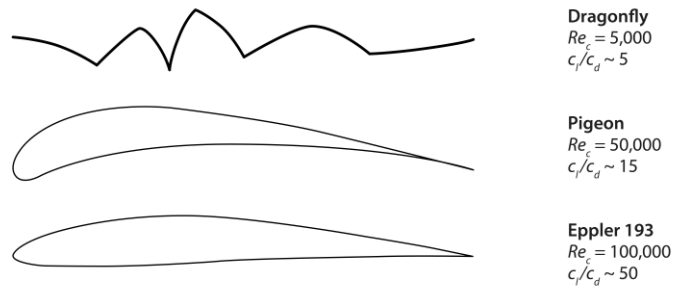
Figure 3. Various representative airfoil shapes versus Reynolds number. 11
