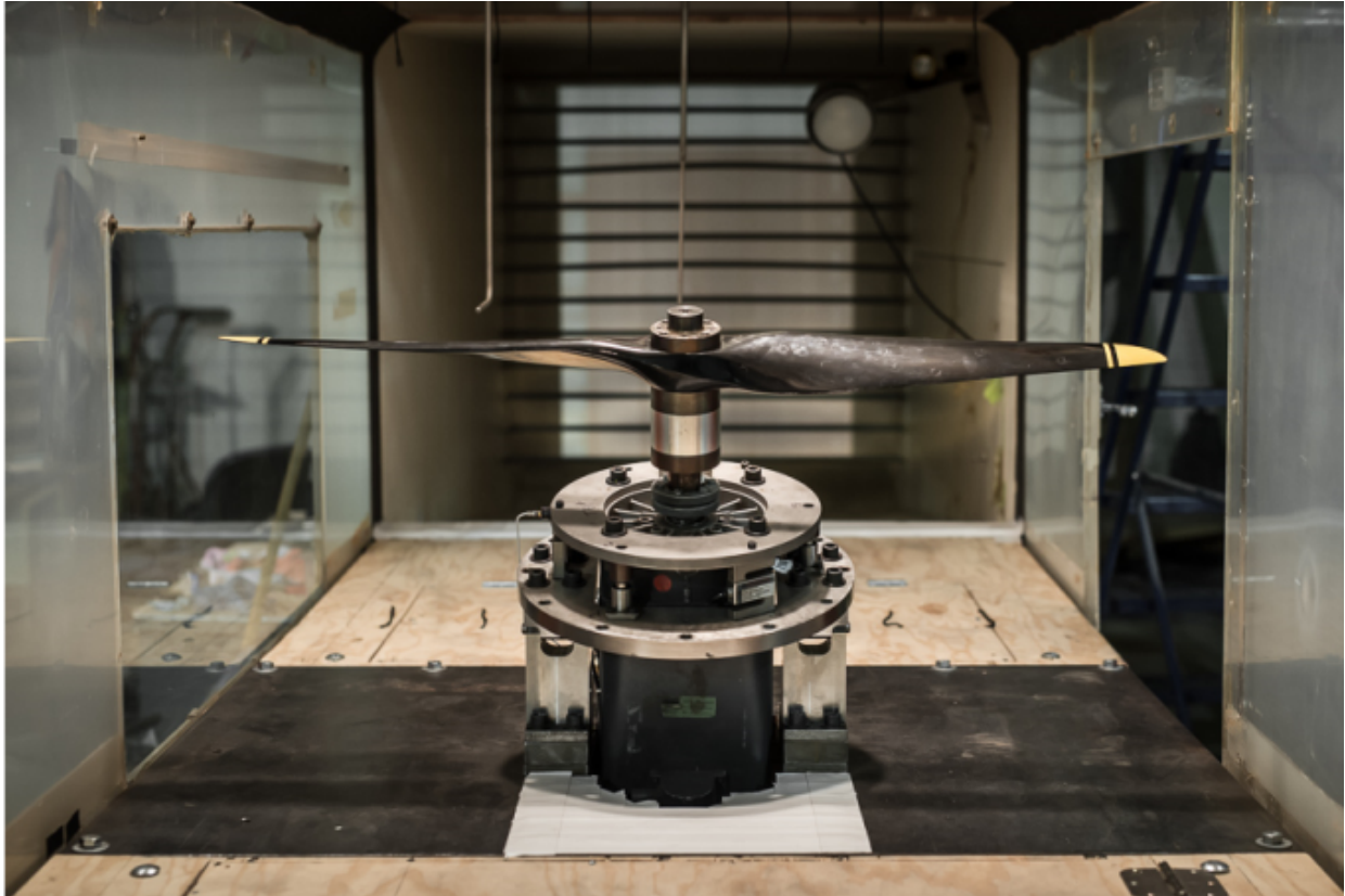
Figure 5. Two-bladed rotor at a -14 -degree shaft angle, looking downstream of the test section.
