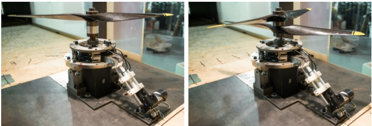
Figure 3. Left and right images show two- and four-bladed rotor configurations tested in the MARSWIT test section, respectively.
