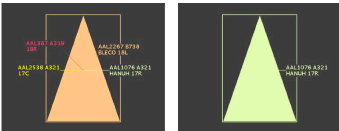
Figure 4.20. Flights by Line-of-Flight: Unselected to show current and future flights (left) and selected to show only the current flight (right).
