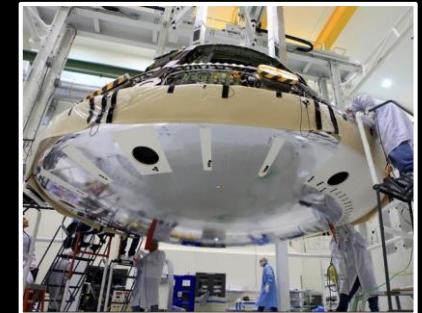
3-D Multi-functional Ablative TPS (3-D MAT) enabling Orion Lunar return
