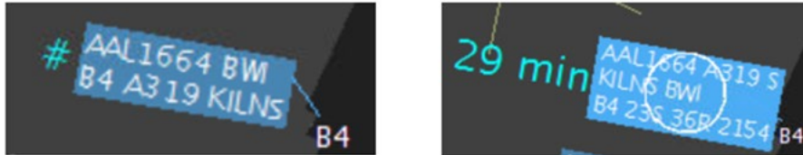
Figure 8.9. “Uncertain” or “Hashtag” flight (left). When pilot calls, click hashtag to see advisory (e.g., 29 min) (right).
