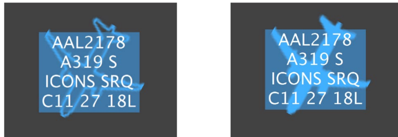
Figure 4.30. Departure flight: Not tracked by surveillance displayed as a hollow flight icon (left) and tracked by surveillance displayed as a solid flight icon (right).
