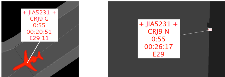
Figure 4.14. Medical emergency examples: Flight icon and attached data tag (left) with red text and red plus signs (+). Flight strip tethered to gate (right).
