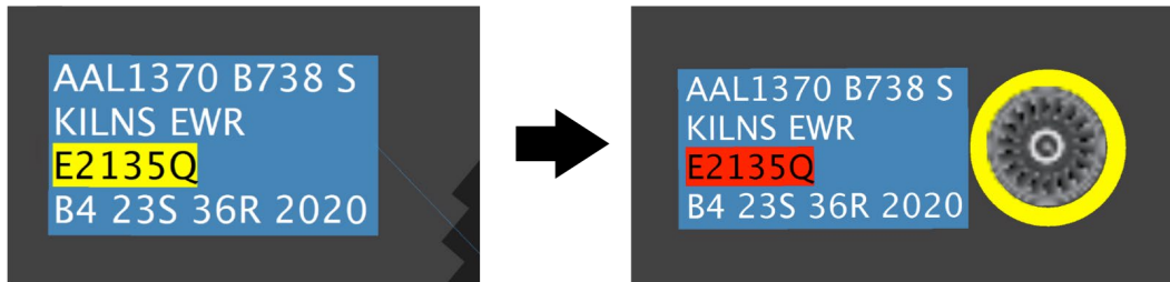
Figure 5.9. When a flight subject to both an EDCT (19:49 UTC, in this example) and an APREQ pushes back without having first contacted ATC to obtain its APREQ time, the field turns red.
