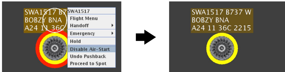
Figure 4.29. When “Disable is Air-Start” is selected from the right-click menu (left), the red circle around the engine icon is removed (right).
