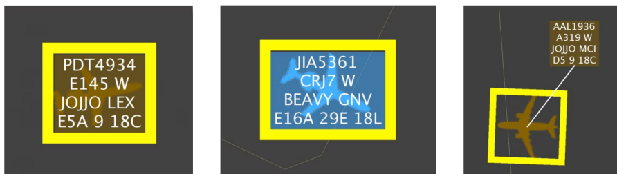
Figure 4.53. Departure flights holding in a hardstand are shown with a yellow border.
