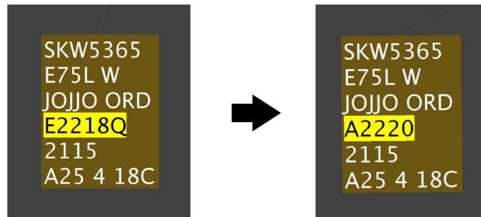
Figure 5.8. When a flight is subject to both an EDCT and an APREQ, the EDCT (22:18 UTC, in this example) is followed by a “Q” -- until the APREQ time is available. Once negotiated, only the APREQ time (22:20 UTC, in this example) is displayed on the flight strip (right).
