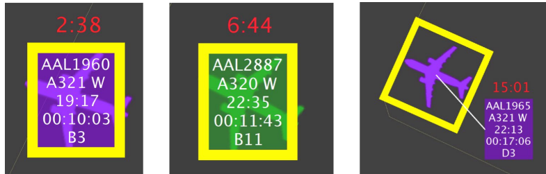
Figure 4.54. Arrival flights holding in a hardstand are shown with a yellow border and an automatic hold timer (red).
