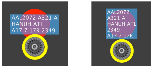
Figure 4.58. Long On Board (LOB) indicators displayed in the pushback/spool-up state (e.g., red indicators = 120+ minutes).
