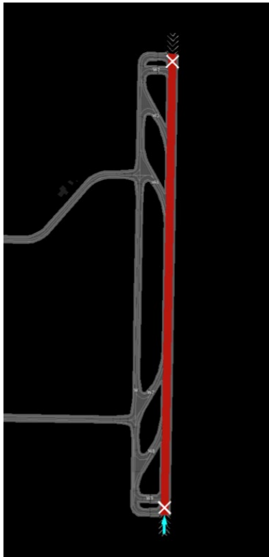
Figure 3.50. Runway closure: Closed runways are shown in red in a white “X” at each end.
