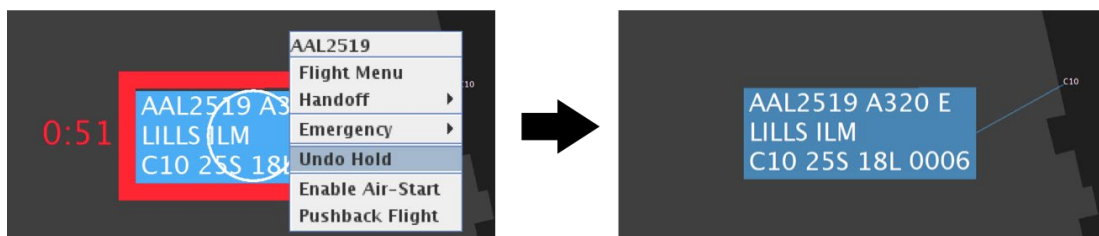
Figure 4.19. Right-click menu with “Undo Hold” selected (left). Red border and accompanying timer are removed from the flight strip (right).
