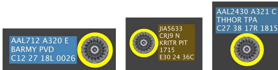
Figure 4.22. Examples of flight strips with attached engine icons in the pushback/spool-up state.
