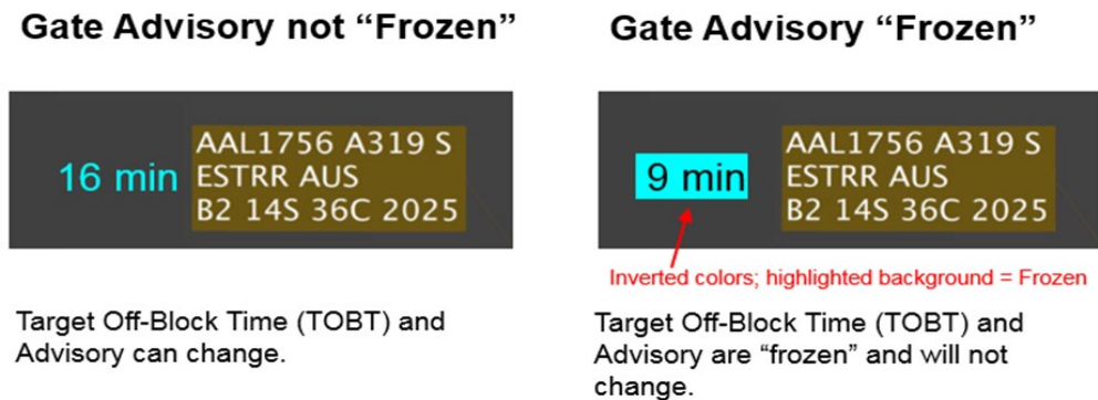
Figure 8.2. Once the TOBT and TMAAT are “frozen”, advisories are displayed as black text highlighted in cyan.
