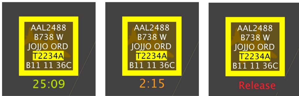
Figure 5.16. TMI-flight holding in hardstand. The light green timer is counting down to the TMAT (left). At 3 minutes prior to the TMAT, the timer turns orange (middle). When the flight should be released from the hardstand, “Release” is shown in red.
