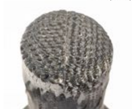
IHF 3": Hot Wall Heat Flux: 3600 W/cm 2 Pressure: 5.3 atm
