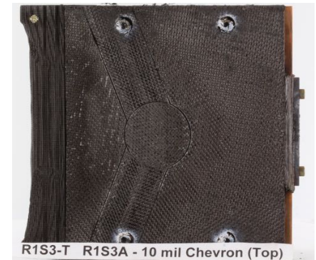
R1S3-T R1S3A - 10 mil Chevron (Top) AEDC Shear Testing: Hot Wall Heat Flux: 1200 W/cm 2 Pressure: 2.9 atm Shear: ~4000Pa
