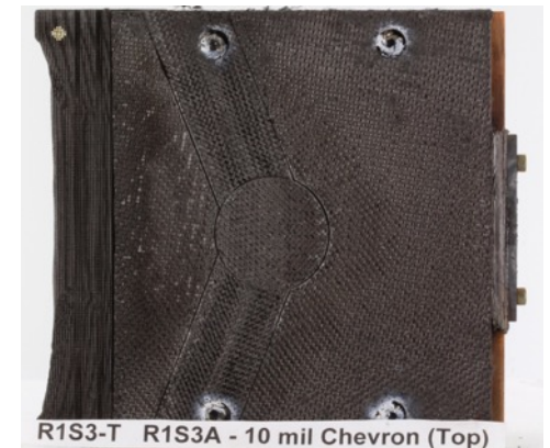
AEDC Shear Testing: Hot Wall Heat Flux: 1200 W/cm 2 Pressure: 2.9 bar/Shear: ~4000Pa
