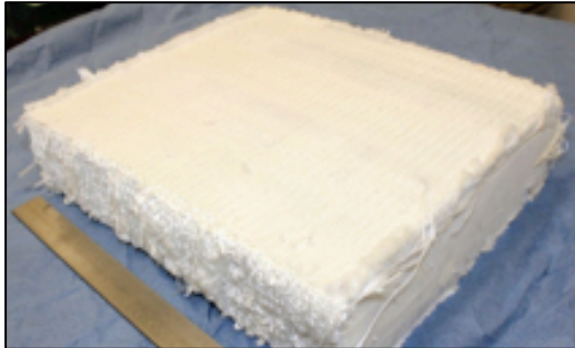
3D, Woven Quartz Fiber Preform
