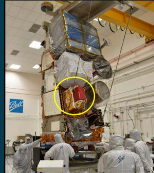
Sensor B NOAA Advanced Technology Microwave Sounder (ATMS) 75kg, 100W, $$$$
