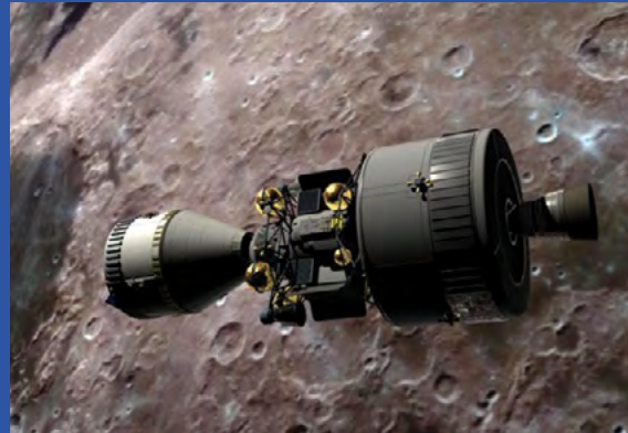
The DASH lander mated to the Orion Crew Exploration Vehicle in Low Lunar Orbit.
