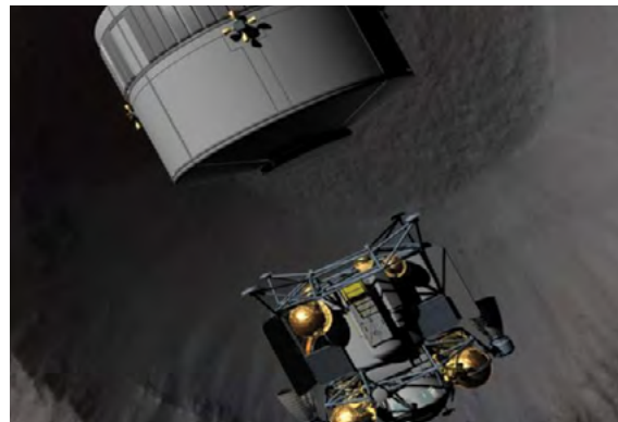
The Retro Module separates from the Lander Module and Payload Module and impacts the surface over 3 km (1.9 mi) downrange of the landing site.
