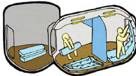
Wall liner installation.
