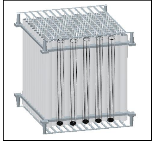
Figure 16: Preliminary assessment of an ESP geometry to support ISRU on Mars
