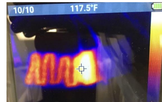
IR thermal image of preliminary heating pad construction: Heat distribution dependency on CNT stitch spacing
