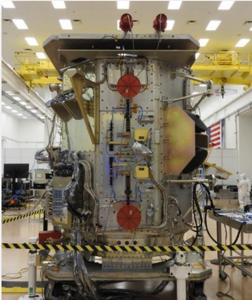
Landsat 9 spacecraft bus being assembled at Northrop Grumman Innovation Systems in Gilbert, AZ
