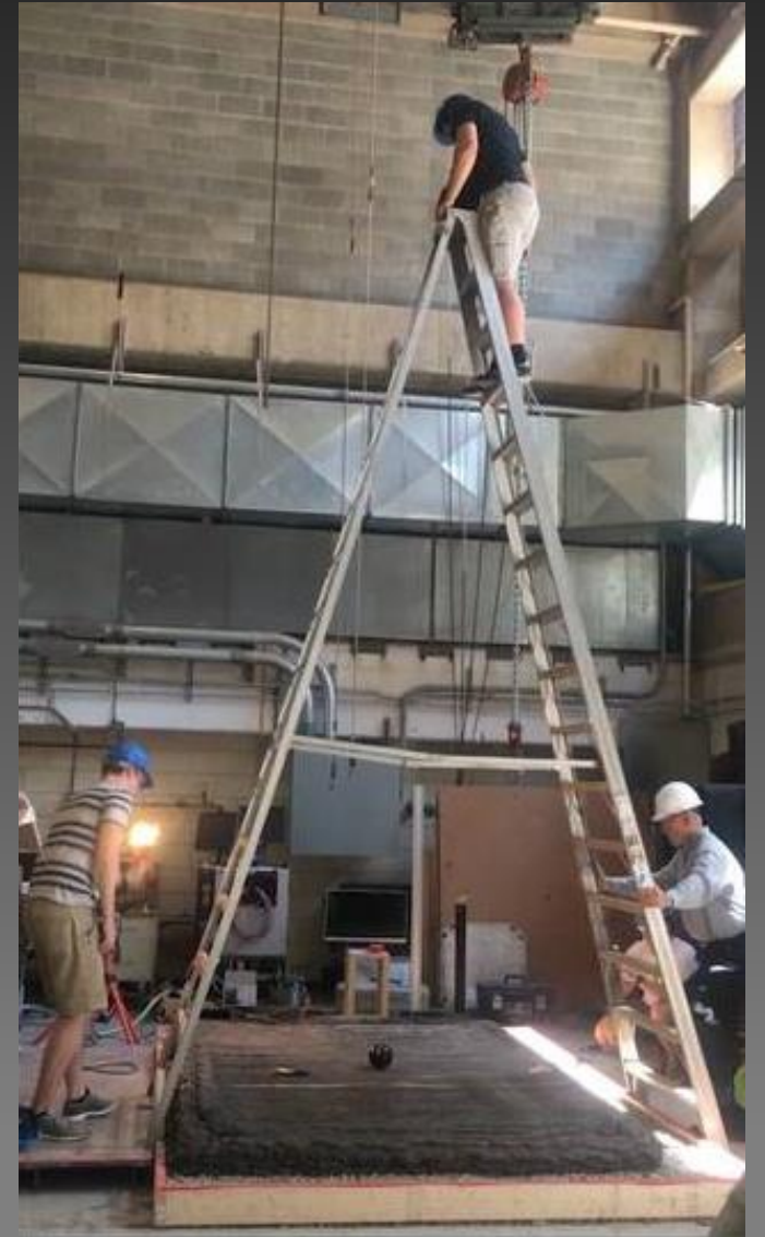
Penn State won second place in this level of NASA's 3D-Printed Habitat Challenge. Pictured above is a shotput drop on the foundation to assess its impact resistance.
