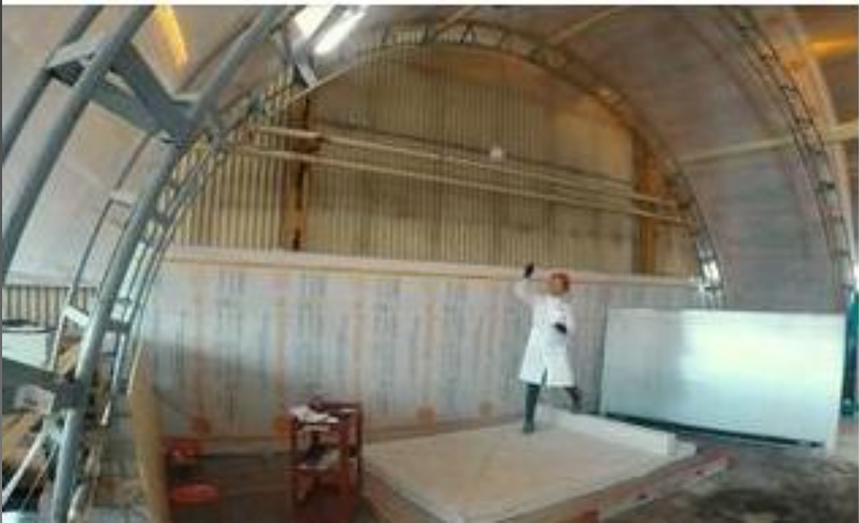
Team SEArch+/Apis Cor of New York won first place in this level of NASA's 3D-Printed Habitat Challenge. The team is pictured above dropping a shotput on their foundation to simulate a meteor strike.
