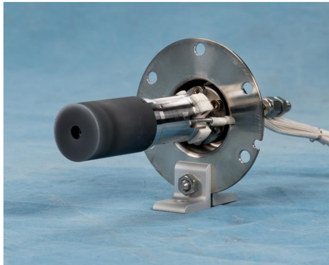
Figure 2. The Mark II cathode, a 25-A class barium oxide hollow cathode developed for the HERMeS Hall Thruster.
