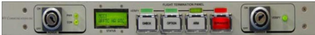
Figure 7.5-6. New FTS Panel, Detail
