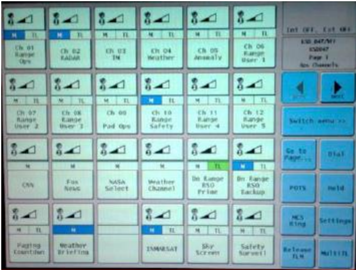
Figure 7.5-2. Touchscreen Used on Range Safety Console MOVE Panel
