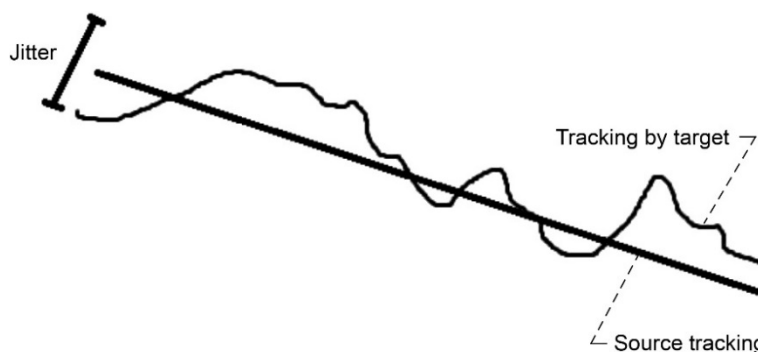
Figure 2.—Time-dynamic misalignment of antenna tracking adapted from Reference 3.
