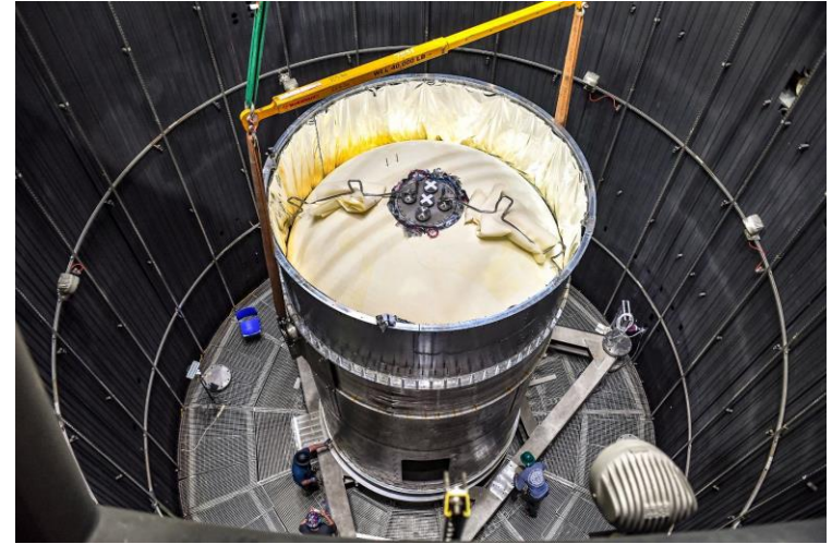
eCryo SHIIVER – liquid hydrogen vapor cooling test in the ISPF facility. (4 meter LH2 PV)
