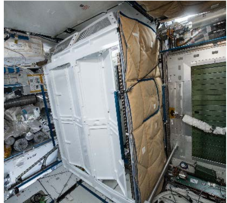
Double Toilet Stall Deployed on ISS
