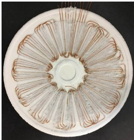
optimized fabrication process for wire-embedded stator
