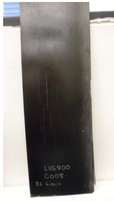
Test article toughened with thermoplastic polyurethane veil between plies
