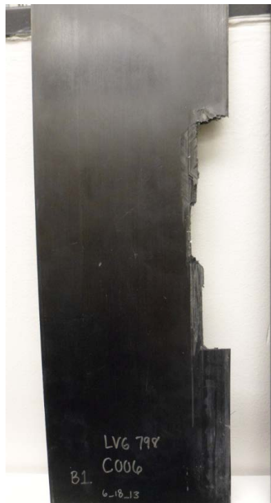
Baseline IM7/8551-7 test article leading edge damage after impact
