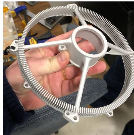
integrated airfoil-shaped cooling fins into motor housing
