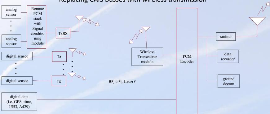
**Replacing CAIS Busses with wireless transmission**
