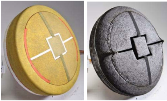
Fig. 25. PICA gap and seam testing (2008) with different seam materials [33]
