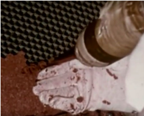
Fig. 9. Insertion of the Apollo ablative material Avco 5026-39G into individual honeycomb cells by “gunning” [10]
