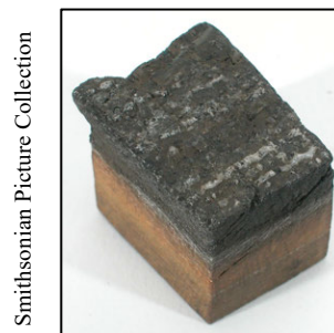
Fig. 2 (b). A small core sample from the heat shield (right) showing char and ablated regions, and cracks [5]
