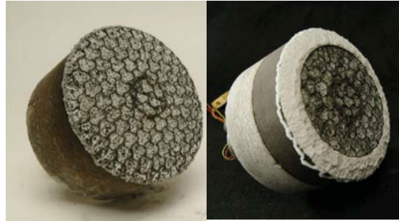
Fig. 22. SLA-561V arc jet tests with stagnation coupons. Left at 150 W/cm 2 and right at 300 W/cm 2 . The appearance differs due to glass vaporization vs glass melt that occurs depending on the local conditions.
