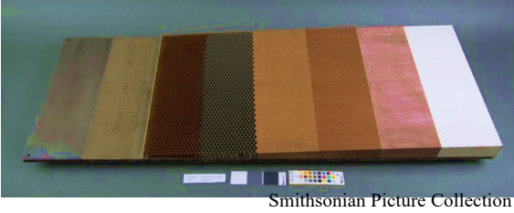
Fig. 8. A demonstration article that illustrates the many steps involved in making avcoat heat shield.
