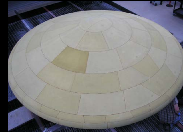
4.5-m diameter tiled ablative heatshield (with in-depth instrumentation!)
