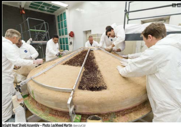
InSight Heat Shield Assembly – Photo: Lockheed Martin 0000 0 of 20
