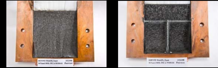
PICA tiles with RTV gap-filler Wedge Tests
