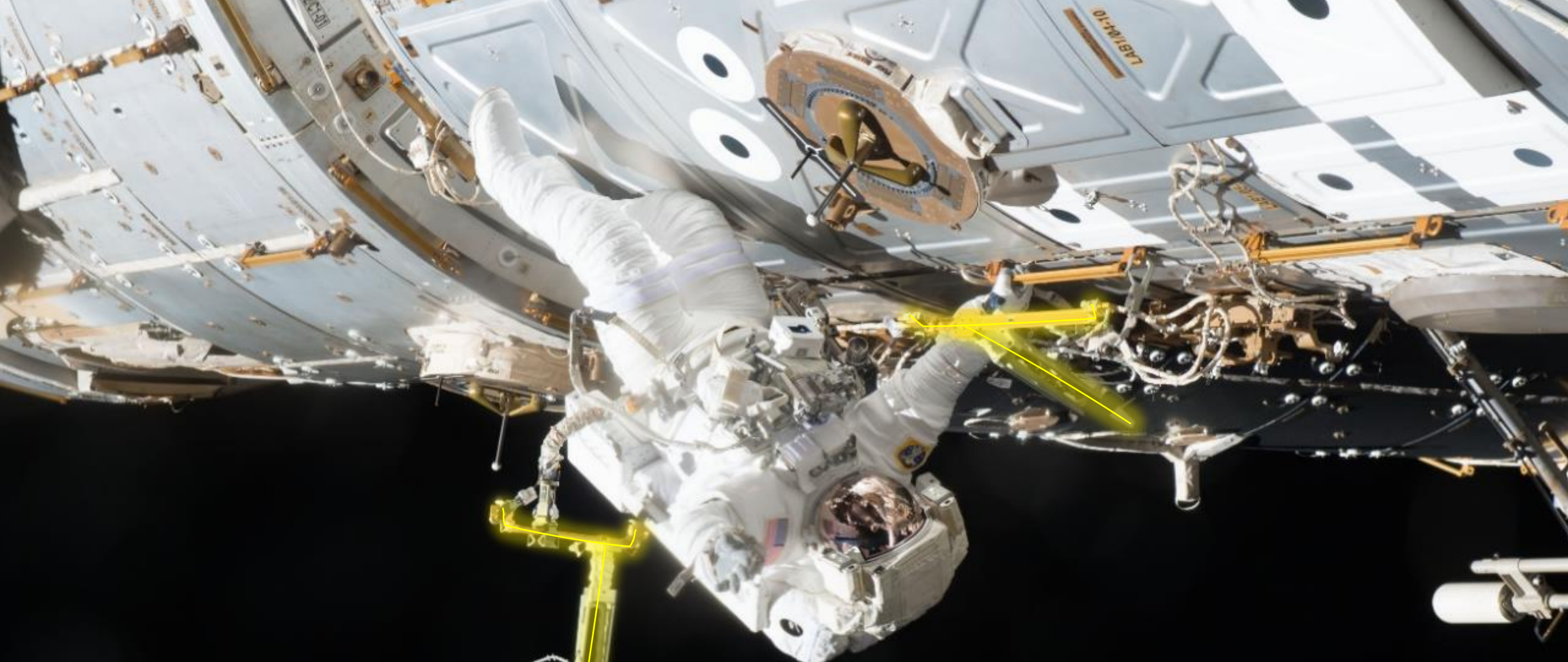
External Wireless US Lab Nadir Antennas
