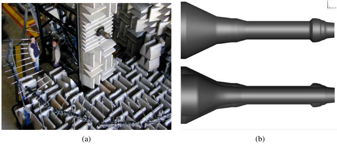
Fig. 2 (a) Picture of the Small Hot Jet Acoustic Rig (SHJAR) in acoustic configuration with 24 microphones centered around the nozzle exit [1]. (b) SMC000 round convergent nozzle used in this study. Drill holes for mounting the nozzle have not been considered in the CFD simulation to simplify the meshing. The nozzle has an exit diameter of 2 inch and a 12 inch straight section between the initial contraction and the nozzle. (bottom) nozzle interior, (top) nozzle exterior.
