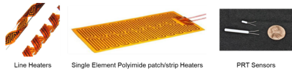
Fig. 7. Thermal control components
