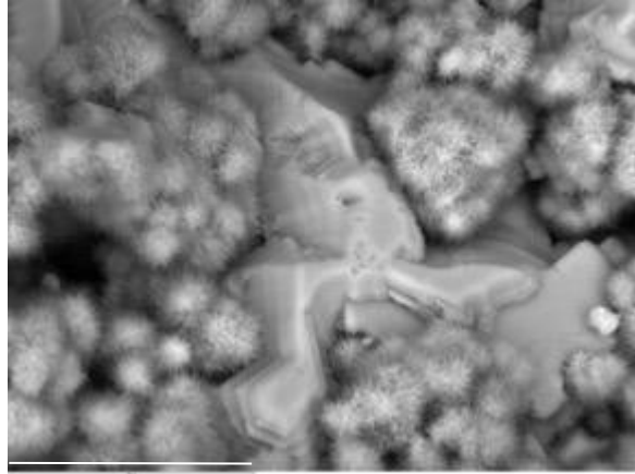
Figure 12: Fractured surface of C 3 S hydrated in μg condition, showing high aspect ratio portlandite with well defined morphology. Scale bar of 25 μm
