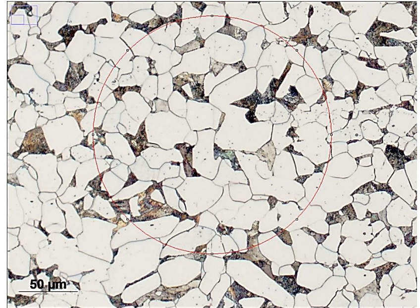
Grain size analysis of low carbon steel using conventional C by ASTM E112-13: Planimetric (Jefferies) Procedure
