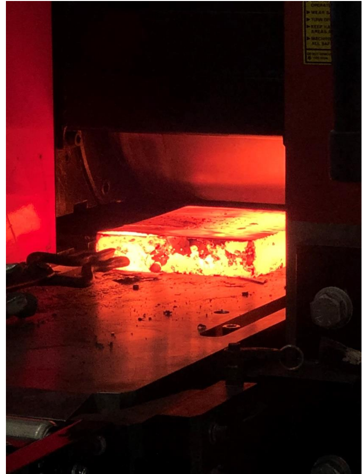
Hot Rolling using In-house Reversing Rolling Mill
