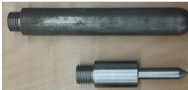
Figure 3-1. Hemispherical impactor (top) and sharp impactor (bottom).
