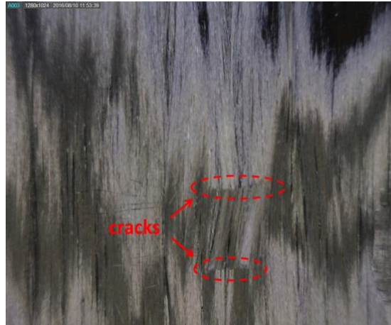
Figure 3-4. Magnified photo of one ply under the microscope.
